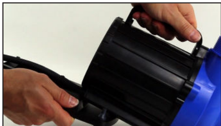
Step 13: Re-fit the base plate.
