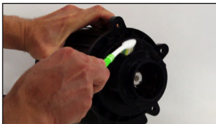
Step 8: Use a brush to clean inside and around the impeller.
